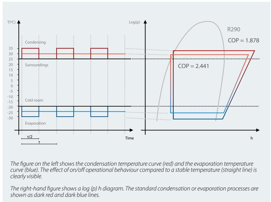
The figure on the left shows the condensation temperature curve (red) and the evaporation temperature curve (blue). The effect of on/off operational behaviour compared to a stable temperature (straight line) is clearly visible.
